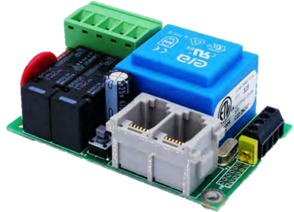
Figure 22. IMC control board
