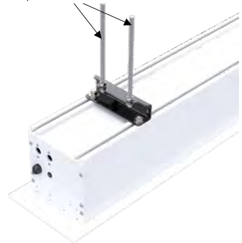
Figure 7. Threaded Rod Mount on top of Cascade unit
