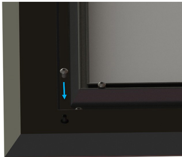
Figure 10: Border trim installed onto frame
