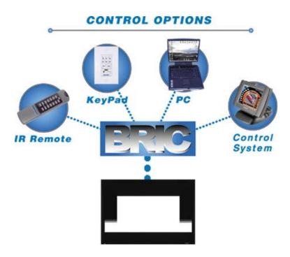
BRIC is available on any Stewart ElectriScreen or ElectriMask system including those with the trap door feature and those units with more sophisticated combined horizontal and vertical masking elements. The BRIC is a self-contained control unit (6-3/8" wide by 7" high) and is mounted within or near the screen itself. BRIC must be specified at time of purchase and ships for easy dealer installation with the BRIC accessory components.
